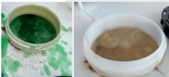
Samples of two different FFFs - Note water absorption creating “sludge” on top of product. Photo Courtesy: LASTFIRE
